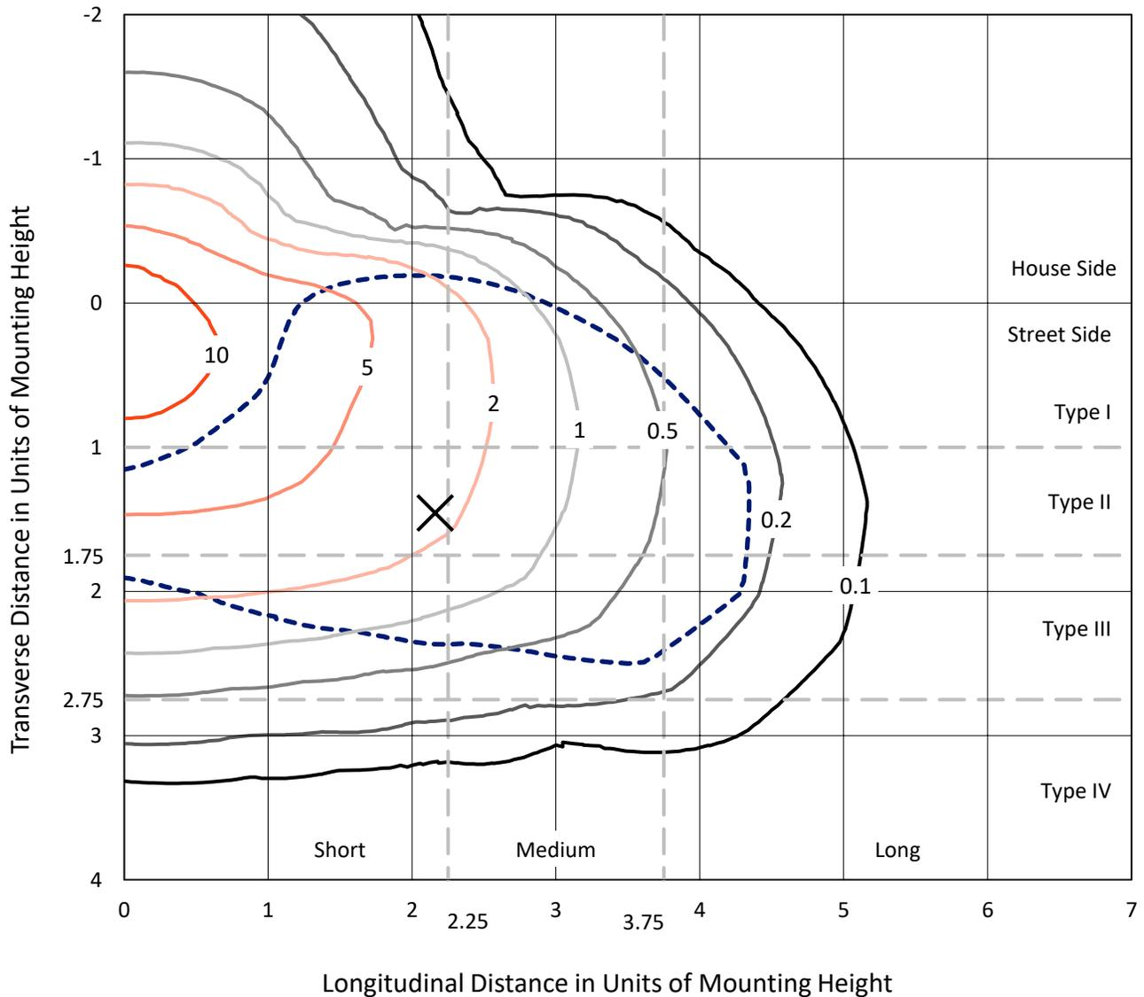
Based on 10 foot mounting height. Maximum calculated value = 11.8 fc
